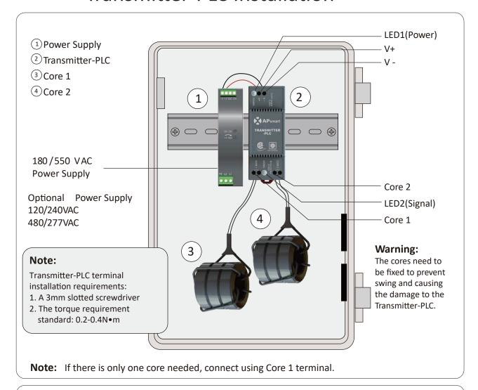
Power supply must be on same AC branch circuit as inverter to meet rapid shutdown requirements.
