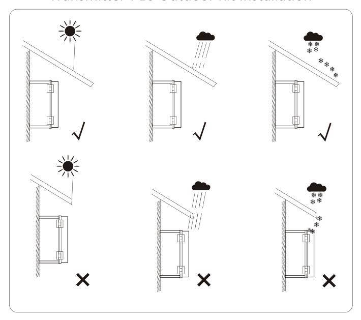
**Warning:** If the Transmitter-PLC-Outdoor Kit is installed outside, it should be protected under shelter from direct sunlight or bad weather conditions (like snow, rain, lightning, etc). Fully shielded installation locations are preferred.
